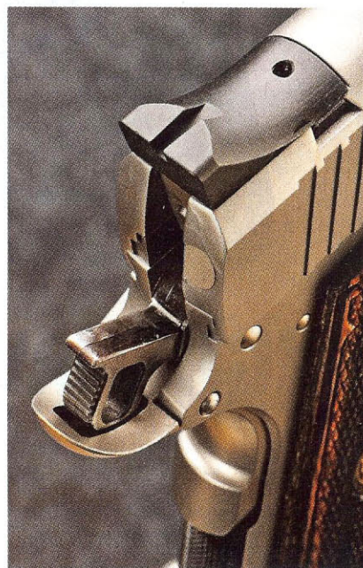
A The 1911TC's robust rear sight is adjustable for windage and was easy to acquire, and the grip safety sports a memory groove.
