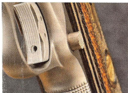
A The extended mag release, along with a beveled mag well, made reloading a snap, and the trigger—which broke at five pounds as it came from the factory—is adjustable.
