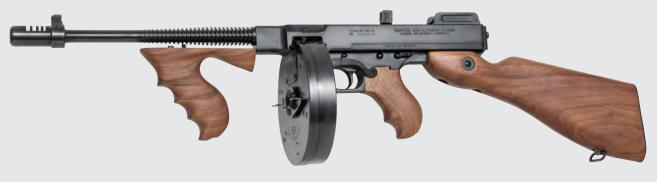
This is the original Thompson design made famous during the 1920's in the hands of gangsters and G-men. Its operation is semi-auto, firing from a closed bolt, and featuring a 10.5" barrel. The frame and receiver are machined from solid steel and the stock is genuine American walnut. The finish is blued steel.
